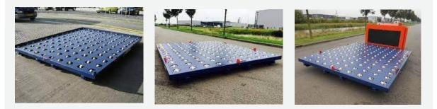
The slave pallet SP-05 is a flexible transport unit consisting of a frame provided with castor wheels which makes a multidirectional transport possible. Combined with a ULD Mover or slave pallets can be used to transport, to store and to build up or break down ULD's. Because of its flexible character, slave pallets are very suitable to expand existing systems temporarily.
