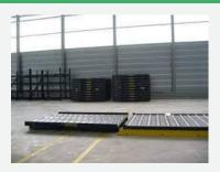
The slave pallet SP-07 is a flexible transport unit consisting of a frame with non-driven conveyor rollers which makes transport possible in 2 directions. Combined with a ULD Mover or Mini Donkey can be used to transport, to store and to build up or break down ULD's. Because of its flexible character, slave pallets are very suitable to expand existing systems temporarily.
