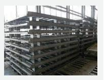
The slave pallet SP-08 is a flexible transport unit consisting of a galvanised frame with non-driven conveyor rollers which makes transport possible in 2 directions. Combined with a ULD Mover or Mini Donkey can be used to transport, to store and to build up or break down ULD's. Because of its flexible character, slave pallets are very suitable to expand existing systems temporarily.
