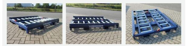
The slave pallet SP-04 is a flexible transport unit consisting of a frame with non-driven conveyor rollers which makes transport possible in 2 directions. Combined with a heavy duty fork-lift truck, the SP-04 can be used to transport, to store and to build up or break down LD3 containers. Because of its flexible character, slave pallets are very suitable to expand existing systems temporarily.
