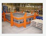
A pallet centring rack is a construction in which empty pallets (96"x 125") can be collected. Through its construction, a pallet centring rack positions aircraft pallets neat on each other.
