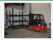
Empty aircraft pallets who are left after handling cargo, can be stored with a forklift in a pallet storage rack.
