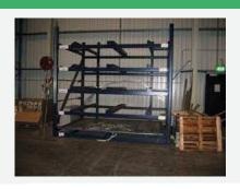
Empty aircraft pallets who are left after handling cargo, can be stored with a forklift in a pallet storage rack.
