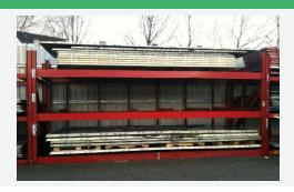
Empty aircraft pallets who are left after handling cargo, can be stored with a forklift in a pallet storage rack.
