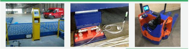
A weighing system can be integrated into a Cargo Handling System at a certain position and assists the handler to determine the weight of an ULD during im- or export, or, during the break up or break down.
